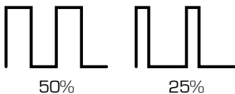
Figure 11-4: Square wave with 50% and 25% duty cycle.
